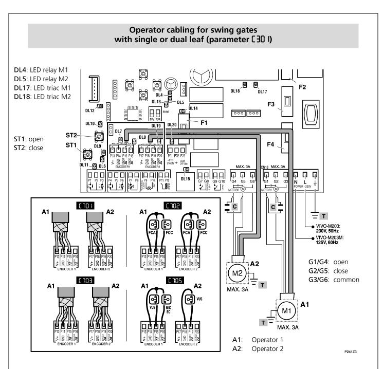
DL7: LED SNG1 (FCA/encoder) A1 DL8: LED SNG2 (FCC/encoder) A1 DL19: LED SNG1 (FCA/encoder) A2 DL20: LED SNG2 (FCC/encoder) A2 ■ The colour of the G1/G4 and G2/G5 cables must be respected in order to correctly programme the turning directions, i.e., the colour of G1 must be the same as for G4 (and G2 the same as G5).
